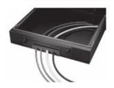
Fits all standard ProLine 100 mm Solid Base gland openings. Can be used in place of standard solid gland plates furnished with 100 mm Solid Base. Adjustable opening for cable entry is foam-lined to maintain a dust-tight seal. Cable Entry Plate is 2,0 mm steel and finished with RAL 9005 textured, black polyester powder paint.
