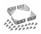
Provides a structural method of bolting a ProLine frame to the floor. Fits all frame sizes. Made of 2.5 mm steel with plated finish. Kit includes four brackets and mounting hardware.
