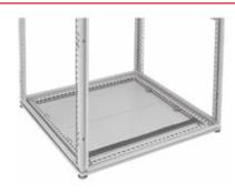
Bottom plate set consists of: bottom plate 1,5 mm painted RAL7035 textured with foam in place gasket; 3 pieces 1,5 mm galvanized gland plates with adhesive foam gaskets; all installation hardware.
