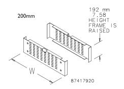
Vented Plinth Base Covers install in the front and rear openings of a standard plinth base in place of Solid Covers. Vented covers allow air to circulate into the enclosure. Vented Plinth Base Covers are available in 100 mm and 200 mm heights. These covers are finished with RAL 9005 black polyester powder paint and include all necessary mounting hardware.
