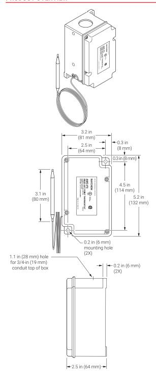
The nVent RAYCHEM AMC-F5 thermostat is designed to control heat-tracing systems used for freeze protection in nonhazardous locations. The thermostat has a fixed set point of 40°F (5°C) and can be used for ambient-sensing or line-sensing. It can be used to control a single heat-tracing circuit or as a pilot control of a contactor switching multiple heat-tracing circuits.
