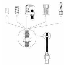
Material: Steel Finish: Electrogalvanized Static Load Safety Factor: 3.5:1
