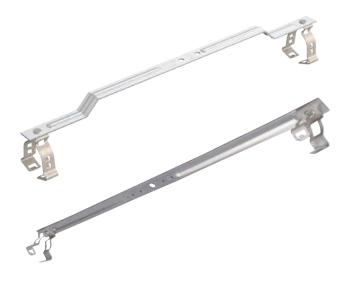
Material: Steel, Spring Steel Finish: Pregalvanized; nVent CADDY Armour The nVent CADDY Combination Box/Conduit Hanger is a fast and secure method to install a wide range of electrical boxes/conduit in overhead installations with a single threaded rod drop. The system is designed to provide greater efficiency in the field with our industry-leading range of nVent CADDY Snap Close Conduit Clamps and innovative nVent CADDY 512X Electrical Box Mounting Clip.
