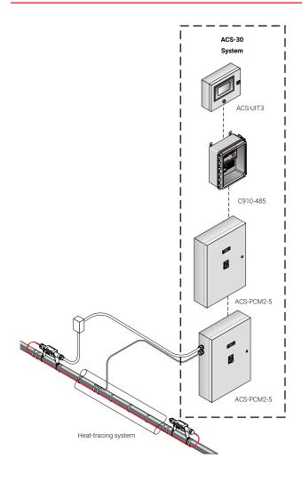
The nVent RAYCHEM ACS-30 Advanced Commercial Control System is a multipoint electronic control and monitoring system for heat-tracing applications. These applications include commercial freeze protection, surface snow melting, roof and gutter de-icing, and flow and temperature maintenance.
