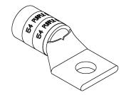
WIRE SIZE: 4/0 MATERIAL: HIGH CONDUCTIVITY COPPER FINISH: TIN PLATED
