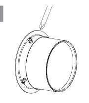
With escutcheon plates held tightly against wall, tighten screws. Repeat process on other side of wall.
