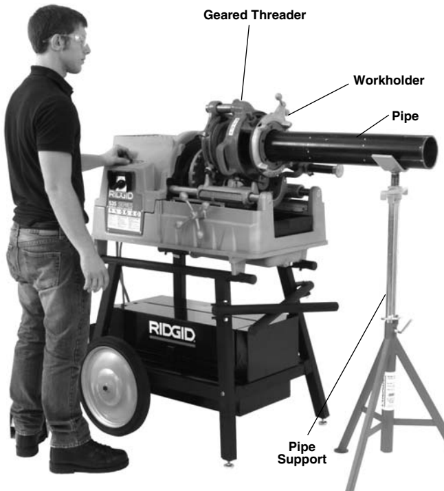
Figure 21 – Operating Position (Close-Coupled Method)
