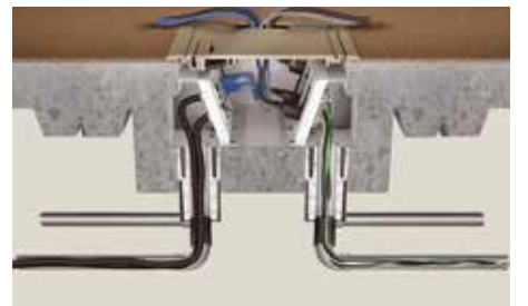
Two Hour Fire Rating – Fire classified for up to two hours and pre-assembled for fast, efficient installation. Just install conduit caps (included), position and secure the box to the desired height in the floor opening.
