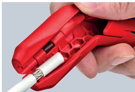
Stripping coax cable sheath
