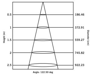
Note: The curves indicate the illuminated area and the average illumination when the luminaire is at different distances.
