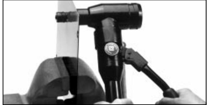
4. Turn the release valve knob clockwise. Rotate driver to best operating position, and then pump lever handle until the punch is completely through the material.
