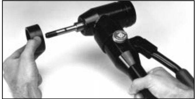
3. Thread 7/16" draw stud tightly into driver. Place the die on the draw stud.
