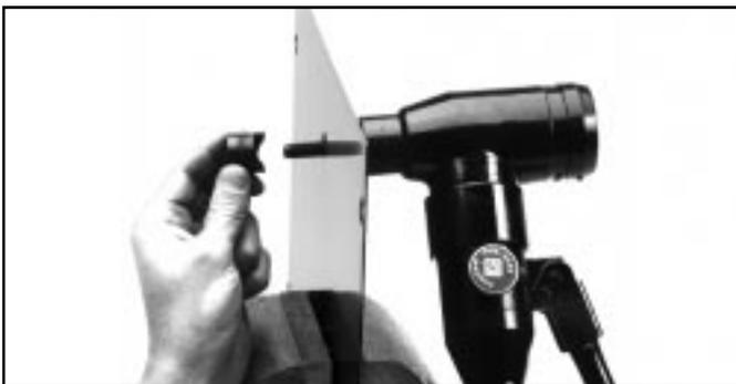
3. Thread 1/2" conduit punch onto draw stud until the punch is tight. Make sure the draw stud threads are fully engaged in the punch.
