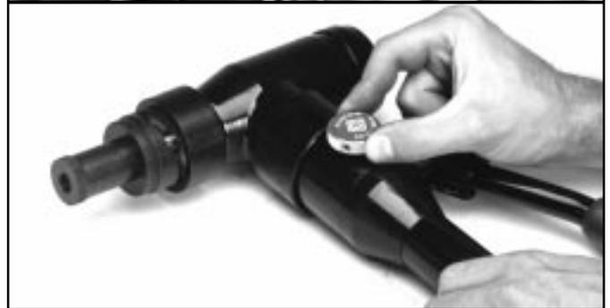
8. Release by turning the release valve knob counter-clockwise.
