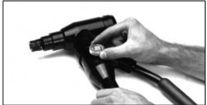
5. Release by turning release valve knob counterclockwise and remove the punch, die, adapter and draw stud.
