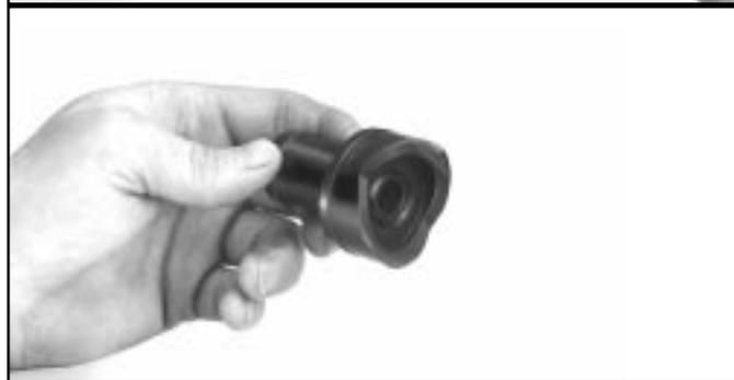
2. Thread the adapter into the punch.
