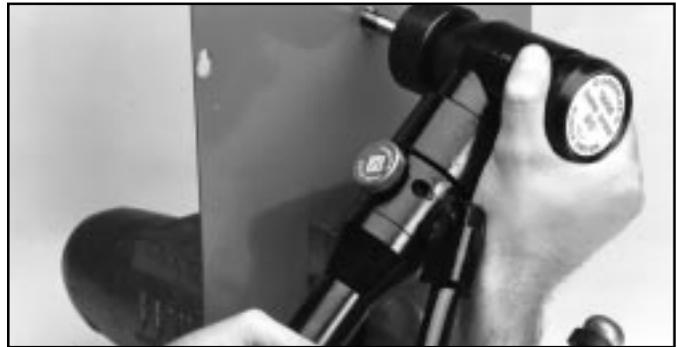
4. Turn the release valve knob counterclockwise, to make sure the draw stud is fully extended. Insert stud through pilot hole.
