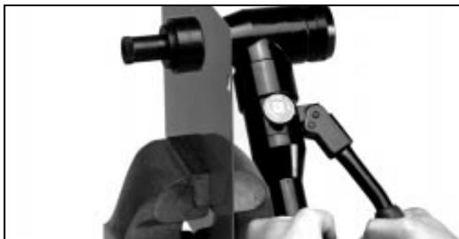
7. Turn release valve knob clockwise. Pump lever handle until the punch is completely through the material.
