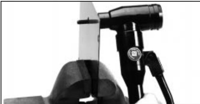
2. Turn the release valve counterclockwise to make sure the ram is fully extended. Install 3/8" draw stud, 3/4" x 3/8" adapter, spacer and 1/2" conduit die and insert into pilot hole.
