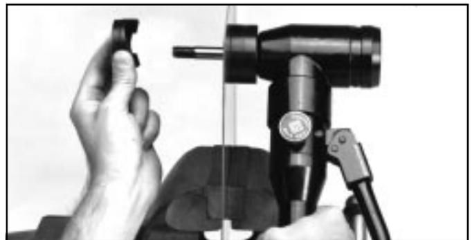
6. Install 3/4" draw stud and select proper size punch and die for desired size hole and repeat steps 4 and 5.
