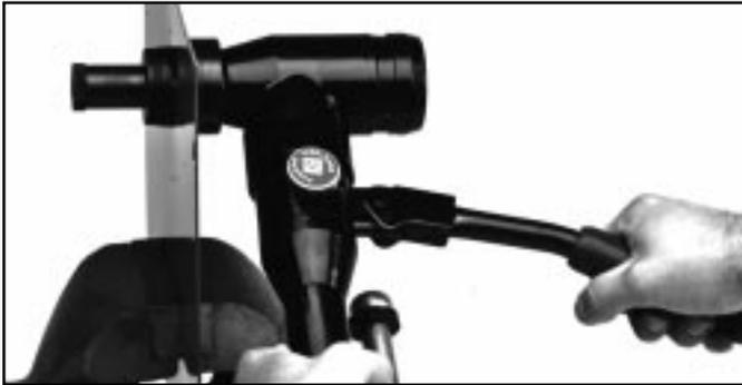
6. Make sure draw stud threads are fully engaged in the adapter.
