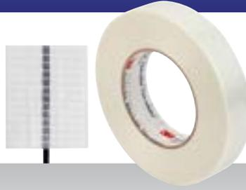
**3M™ Filament Reinforced Electrical Tape 1039** is a more conformable, solvent-resistant tape with an acrylic adhesive. It is commonly used for holding down magnet wire, copper strips (sheets), and insulation materials during the demanding coil winding process. It's also used in lead anchoring, banding of coils, lead tape anchoring, and anywhere tensile strength is needed.
