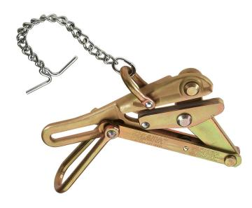
The Klein Tools 1628-16AT Chicago Grip is identical to a Bell-System type H Strand Puller. It is equipped with a chain, toggle and shackle to keep the grip from falling off the cable. All Klein grips are manufactured from custom drop-forged steel that is machined and heat treated for excellent durability. Each grip is individually hand inspected and actuated for proper function. Grips are also rigorously tested and pulled to rated load to ensure the highest quality and reliability.
