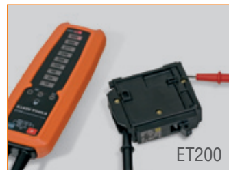
Check Circuit Breaker Continuity
