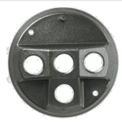
Corrosion-proof round four hole cover. Tough polycarbonate with molded-in color. Fourth hole is perfect for motion sensor mounting. Fits 4" round boxes. Supplied with thick foam rubber gasket. One molded 1/2" close-up plug and (2) stainless steel screws.
