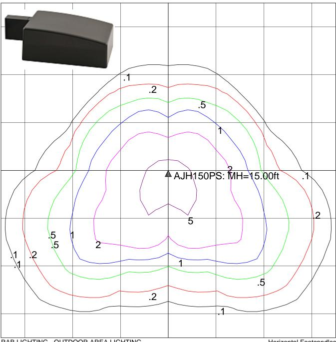
RAB LIGHTING - OUTDOOR AREA LIGHTING LUMINAIRE AJH150PSQ WITH SEMI-SPECULAR REFLECTOR AND CLEAR FLAT GLASS LENS VENTURE 150 WATT PSMH LAMP Horizontal Footcandles
