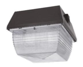
Medium size ceiling mount fixture: 26, 32 and 42 Watt compact fluorescent available. Housing is die cast aluminum with clear vandalproof polycarbonate refractor. Photocontrol, Sensor (CFL 120v only) models available. Lamp supplied.
