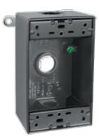
Die cast aluminum with two unique "flex-lugs" for wall or pole mounting of outdoor outlets, switches or floodlights. Ground screw and close-up plugs provided. Cubic capacity is 18.3 cu. inches.
