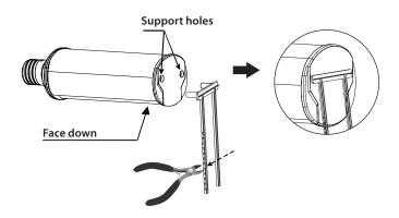
For face-out installation: use the one-legged support and cut to desired length
