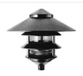
Rugged die cast aluminum 6" diameter housings. Threaded, gasketed clear glass globe for durable weatherproofing and easy relamping. 1" long, 1/2" threaded nipple included for easy mounting. 100 Watt max. Incandescent lamp not supplied. Fluorescent lamp supplied.
