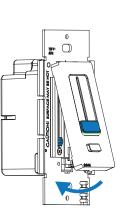
c. Insert face plate back into top housing groove. Position housing slider and brightness (bottom level) and pop on face plate.
