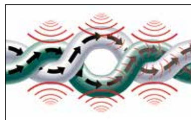
Illustration 1: Example of Non-Bonded-Pair. As cable is stretched and pulled, pairs begin to separate, causing a degradation in signal quality.
