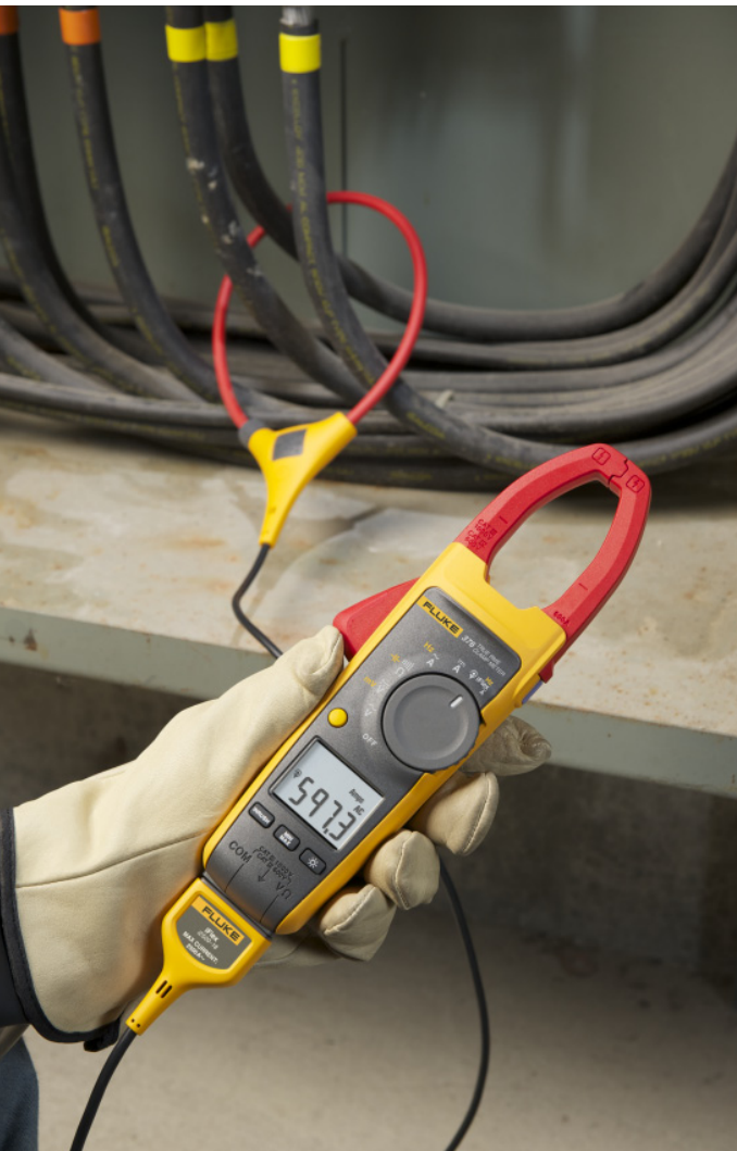
A flexible current probe allows you to measure the current in several conductors at one time—a difficult undertaking using only the clamp jaws.
