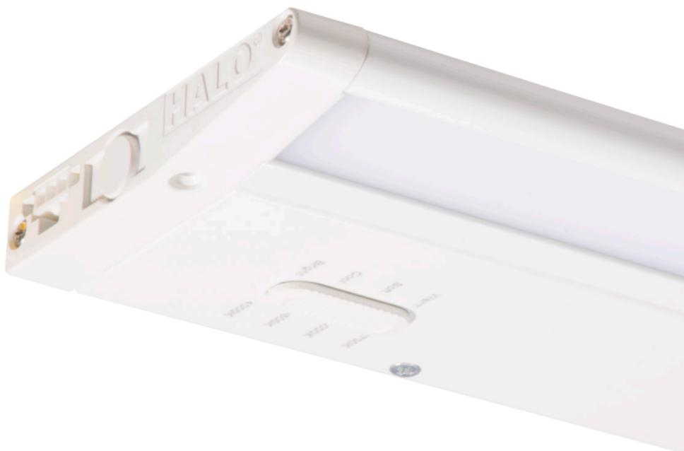
The HU30 has smooth dimming down to 5% using a TRIAC or ELV dimmer. Connector cables in a variety of different lengths make it easy to link multiple units together up to a maximum of 450W. Each unit features an integrated on-off switch and a special optical system provides a smooth beam pattern to minimize pixilation.
