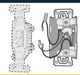
10 Connect the HALO Home Smart Switch (A) using provided wire nuts (B).
