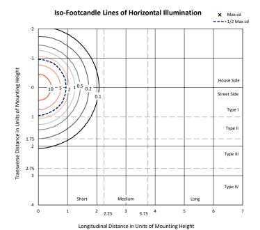
Based on 10 foot mounting height. Maximum calculated value = 14.7 fc Type V - Short - Full Cutoff
