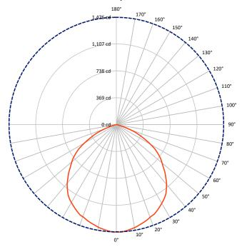
— Vertical Plane Through 67.5-Deg Lateral −−− Horizontal Cone Through 2.5-Deg Vertical
