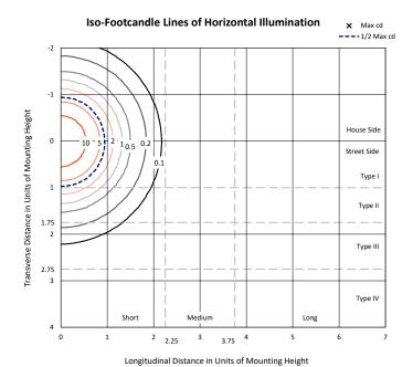
Based on 10 foot mounting height. Maximum calculated value = 18.7 fc Type V - Short - Full Cutoff
