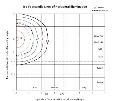
Based on 10 foot mounting height. Maximum calculated value = 10.6 fc Type II - Short - Cutoff
