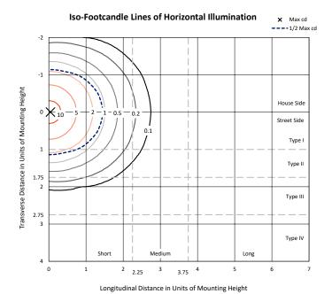
Based on 10 foot mounting height. Maximum calculated value = 12.3 fc Type V - Short - Cutoff
