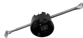
4" round new work non-metallic box with hanger bar assembly 4" diameter x 2-3/16" (102mm x 56mm)
