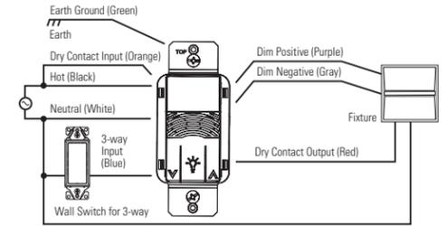
Only one sensor can be used in a 3-way circuit with a switch. The switch will turn on/off the load only at the brightness level selected at the dimmer.
