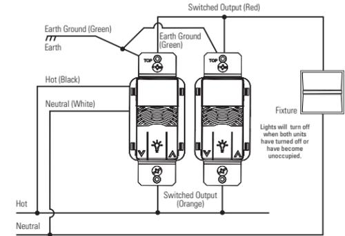
**CAUTION:** If a room is wired for two circuits using two separate hot leads, it is very important to connect only one circuit per relay. Both circuits must be fed from the same phase.
