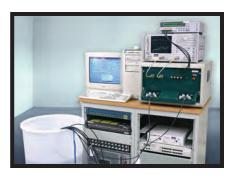
The water bath test is a six-month long test, with the cables fully submerged in water.
