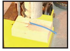
In the cold impact test, after the cable is cooled an aluminum weight smashes against it
