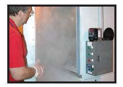
In the cold bend test, the cables were first placed into a cold box.
