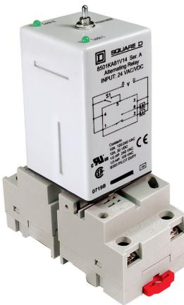
8501 KA alternating relays are designed to minimize pump and motor wear by equalizing run time between parallel components in a multi-pump system. These relays are controlled by an external control switch. This switch may be any type of contact closure; for example, the contacts of a timing relay or the closure of a float switch. The 8501 KA relays also have a toggle switch that allows the operator to lock one side of the duplex system, preventing alternation.
