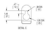
Dimensions shown in inches and millimeters ( ). Dimension shown accurate to  $\pm\,\,1\!\!/\!_{e}$  inch.
