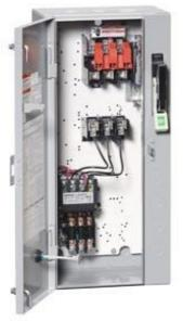
Non-reversing motor starter, Size 0, Three phase full voltage, Amb compensate bimetal OLrelay Contactor amp rating 18Amp 110V 50HZ / 120V 60HZ coil, Combination type, 30Amp fusible disconnect 30 Amp /250V fuse clip, Enclosure NEMA type 1, Indoor general purpose use, Standard width enclosure
