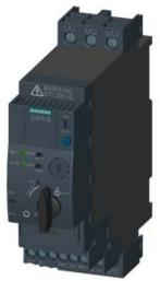
SIRIUS, COMPACT STARTER, DIRECT STARTER 690 V, 110 ... 240 V AC/DC, 50 ... 60 HZ, 0.32 ... 1.25 A, IP20, CONNECTION MAIN CIRCUIT: SCREW TERMINAL, CONNECTION AUXILIARY CIRCUIT: SCREW TERMINAL
