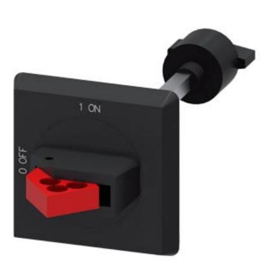
Door-coupling rotary operating mechanism IP64 for circuit breaker Size S00...S3, 130 mm shaft as 3RV29260B, but for switch installation rotated by  $90^\circ$ , same position of the cover inscription OFF = left, ON = top
