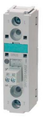
Semiconductor relay, 1-phase 3RF2 Width 22.5 mm, 20 A 48-460 V / 24 V DC screw terminal Instantaneous switching
