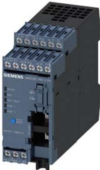
Basic unit SIMOCODE pro V PN, Ethernet/PROFINET IO, PN system redundancy, OPC UA server, Web server, transmission rate 100 Mbps, 2 x bus connection via RJ45, 4I/3O freely parameterizable, Us: 24 V DC, input for thermistor connection Monostable relay outputs, expandable by extension modules
