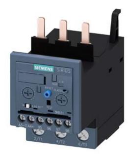
Overload relay 20...80 A Electronic For motor protection Size S2, Class 5E...30E Contactor mounting Main circuit: Screw Auxiliary circuit: Screw Manual-Automatic-Reset Internal ground fault detection
