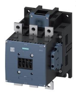
Power contactor, AC-3 300 A, 160 kW / 400 V AC (50-60 Hz) / DC operation 110-127 V UC Auxiliary contacts 2 NO + 2 NC 3-pole, Size S10 Busbar connections Drive: conventional screw terminal NEMA version
