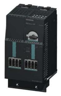
RS1E-X for ET200S High Feature reversing starter Setting range 2.4...16 A Mechanical switching Electronic protection AC-3, up to 7.5 kW / 400 V expandable for Brake control module 2DI module 2DI module Motor starter ES Circuit breaker signaling parameterizable DPV 1-capable PROFIENERGY-capable to PN
