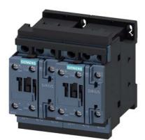
reversing contactor assembly, AC-3e/AC-3, 25 A, 11 kW / 400 V, 3-pole, 110 V AC, 50 Hz / 120 V, 60 Hz, screw terminal, electrical and mechanical interlock, auxiliary contacts: 2 x 1 NO
