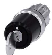
key-operated switch Siemens, 22 mm, round, metal, shiny, lock number SSG10, with 2 keys, 3 switch positions I-O-II, latching, actuating angle  $2x45^{\circ}$ , 10:30h/12h/13:30h, key removal I+II, with laser labeling, upper case
