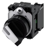
Selector switch, illuminable, 22 mm, round, plastic, white, selector switch, short, 2 switch positions O-I, latching, 10:30h/13:30h, with holder, 1 NO, screw terminal, with laser labeling, upper case and lower case, always upper case at beginning of line
