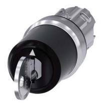
Key-operated switch IKON, 22 mm, round, metal, shiny, special lock, with 2 keys, 3 switch positions I-O-II, latching, actuating angle 2x45°, 10:30h/12h/13:30h, Key removal I+O+II
