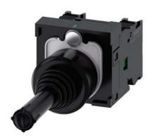
Coordinate switch, 22 mm, round, plastic, black, 2 switch positions, vertical, momentary contact type, without mechanical interlocking in O position, with holder, 1 NO, 1 NO, screw terminal, with laser labeling, inscription or symbol Customerspecific selection with SIRIUS ACT configurator (CIN)
