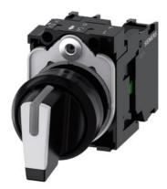
Selector switch, illuminable, 22 mm, round, plastic, white, selector switch, short, 3 switch positions I-O-II, latching, 10:30h/12h/13:30h, with holder, 1 NO, 1 NO, screw terminal, Z=20-unit packaging
