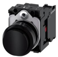
Pushbutton, 22 mm, round, plastic, black, pushbutton, raised, momentary contact type, with holder 1 NC, screw terminal, Z=20-unit packaging
