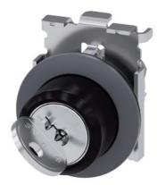
RONIS key-operated switch, 30 mm, round, Metal, matte, front ring for flush installation, lock number SB30, with 2 keys, 2 switch positions O<1, momentary contact type, Actuating angle 45°, 10:30h/12h, key removal O, possible special locks: SB31, 421, 455, with laser labeling, upper case
