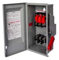
Siemens Low Voltage Circuit Protection Heavy Duty Safety Switches. Type: ENCLOSED, SAFETY SWITCH Std: CUL V. Rating: 600V A. Rating: 200A Wattage: 4W No. Of Poles: 4P F. Rating: 60Hz Action: SINGLE THROW Material: STEEL Enclosure: TYPE 1. 2-3 point mounting holes. O. Cycles: 8000 O. Temperature: (-20F-120F) AMBIENT TEMPERATURE Environmental Conditions: INDOOR
