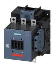
power contactor, AC-3e/AC-3 185 A, 90 kW / 400 V AC (50-60 Hz) / DC Uc: 110-127 V 3-pole, auxiliary contacts 2 NO + 2 NC permanently mounted drive: conventional main circuit: busbar control and auxiliary circuit: screw terminal
